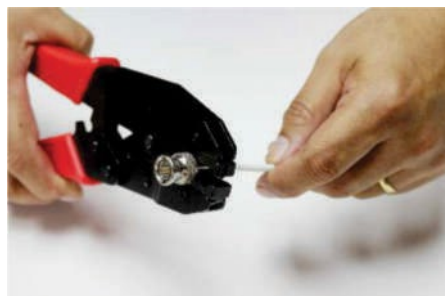
Crimp with the help of hexagonal pliers.
