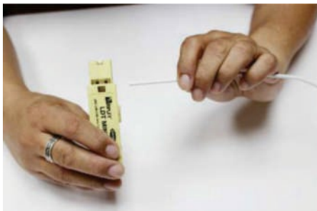
Strip the cable using the RIPLEY stripper.
